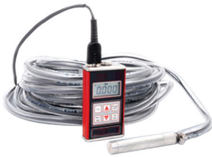
Figure 1. Underwater-capable UT unit with long transducer cable.
