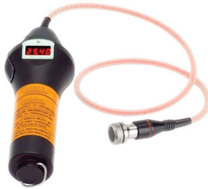
Figure 2. Diver held UT unit. Note display visible to diver.
