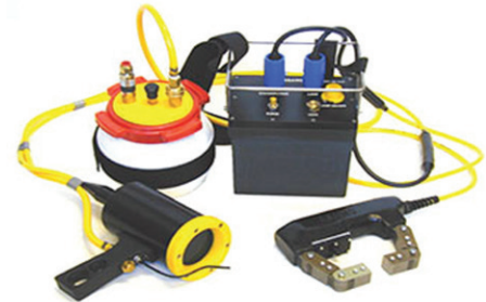
Figure 3. Underwater MT system, with diver-held yoke and lamp.
